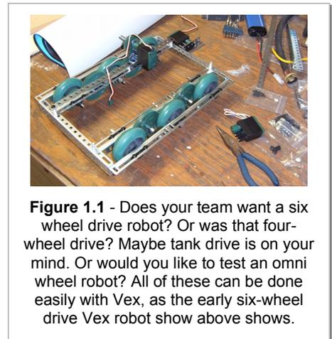
Figure 1.1 - Does your team want a six wheel drive robot? Or was that four-wheel drive? Maybe tank drive is on your mind. Or would you like to test an omni wheel robot? All of these can be done easily with Vex, as the early six-wheel drive Vex robot show above shows.
