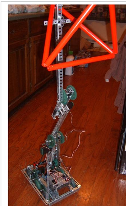
**Figure 1.4** – In the above picture, the elevator is a single stage with roughly 11 inches of travel. The arm is built off the upper portion of the elevator, and can rotate about 270°. As with the rest of the robot, everything is 100% Vex only parts. But wait, is that a real 1:3 scale tetra?
