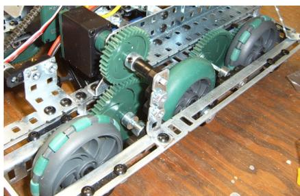
Figure 1.2 - Later on, omni wheels were tried out on my Vex robot. With a full size robot, this would mean ordering omni wheels online (or fabricating your own), waiting for them to arrive, and installing them. However, with Vex, wheel and gearing combinations can be changed in minutes.
