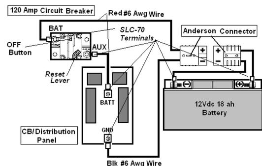
**12Vdc Battery & Main Power Connections**
